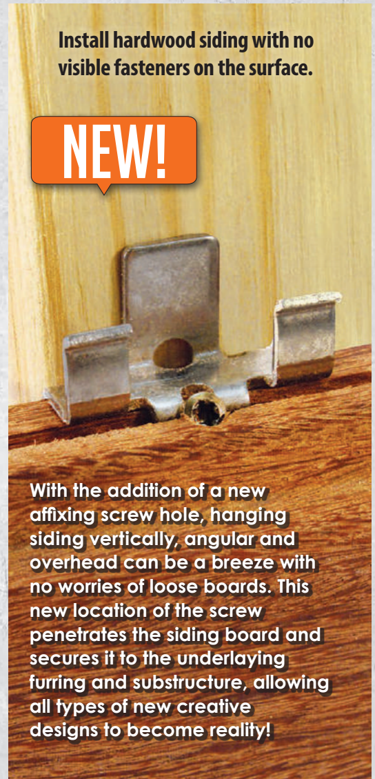
SCREW LOCATION IF HANGING SIDING ON THE VERTICAL, ANGULAR, OR OVERHEAD
