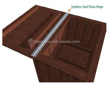
A piano hinge is best suited to this type of lid as it runs the full length which adds stability to both the lid and box side. The hinge is cut ½ inch less than the length of the box. This hinge sits directly on the surface and does not need recessing down.
