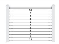
Follow the recommended tensioning sequence below to ensure proper installation and to achieve optimal results.
