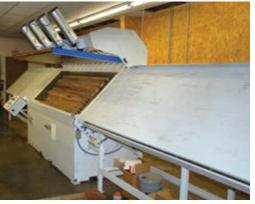
Our Radio Frequency Gluing Machine allows us to produce edge-glued panels faster and with stronger glue joints than traditional gluing methods.
