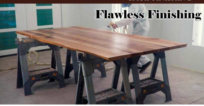
The new spray booth at our Sarasota mill makes us a true one-stop shop for all your wood slab needs. A spray booth sucks the dust and overspray out of the room, keeping debris off the slab surface and preventing rough spots. It allows us to efficiently apply a professional factory finish to any slab.
