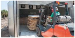
Loading our dehumidification kiln, which has a capacity of 14,000 bd. ft.
