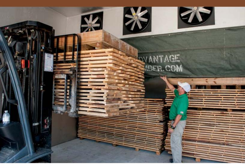
temperature, pressure, and humidity to yield the best lumber with consistent moisture content. This selection of kilns allows us to produce both small custom orders for retail clients and large truckload volumes for wholesale orders.
