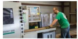
Each deck board is run through our European-engineered molder to create the perfect pregrooved or siding profile every time.
