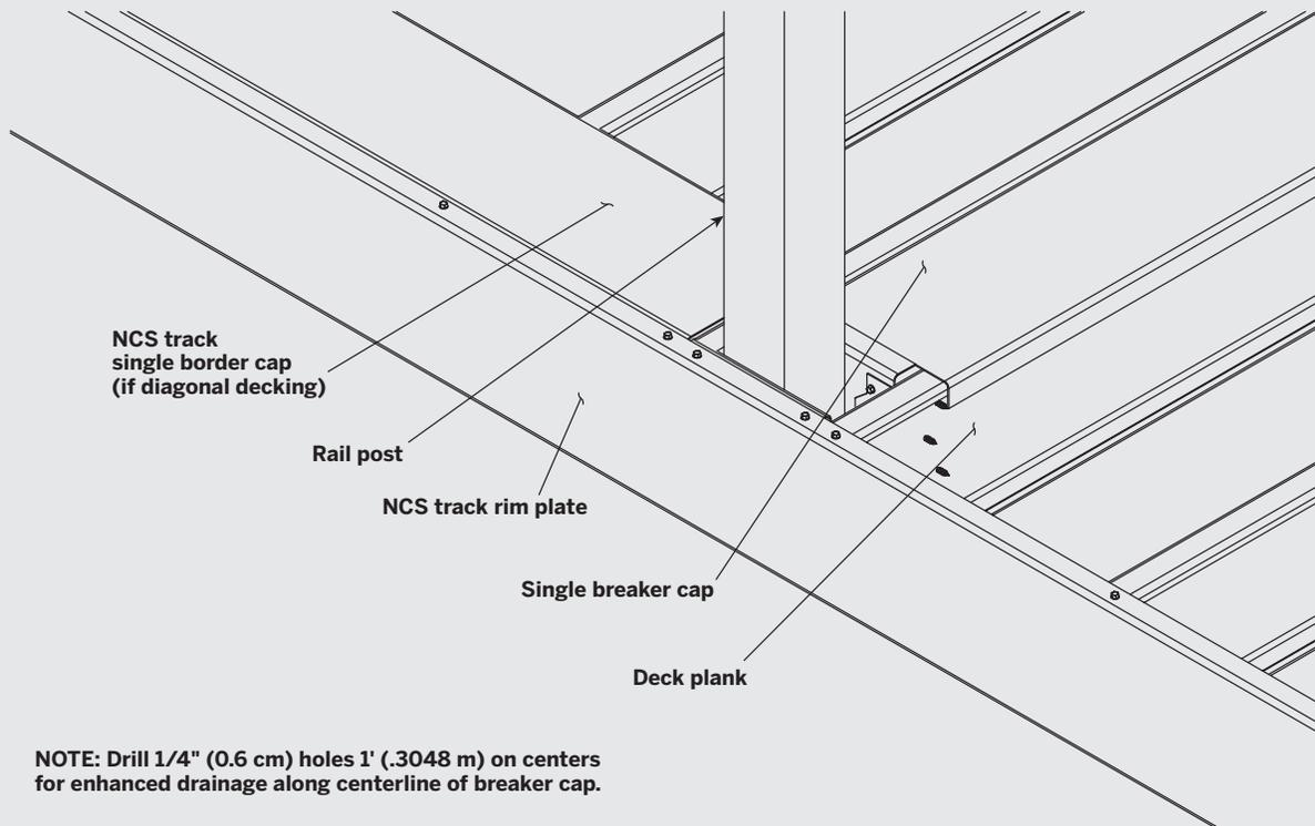
NOTE: Drill 1/4" (0.6 cm) holes 1' (.3048 m) on centers for enhanced drainage along centerline of breaker cap.
