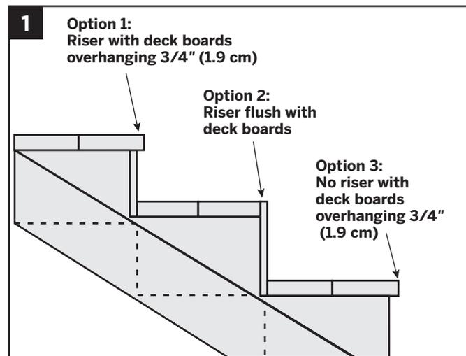
1. Install the deck boards as required by local code. Check with your local building code inspector for requirements.
