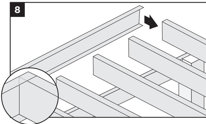
8. Position track as a rim plate. Fit existing joists within the flanges of the track.
