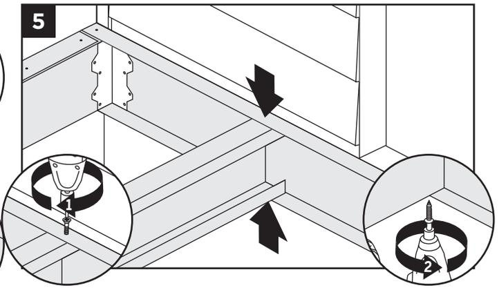
5. Fasten top and bottom of joist and track. Screw joist to track from above and below with required fasteners. See *Required Fasteners chart on page 6, column A*.
