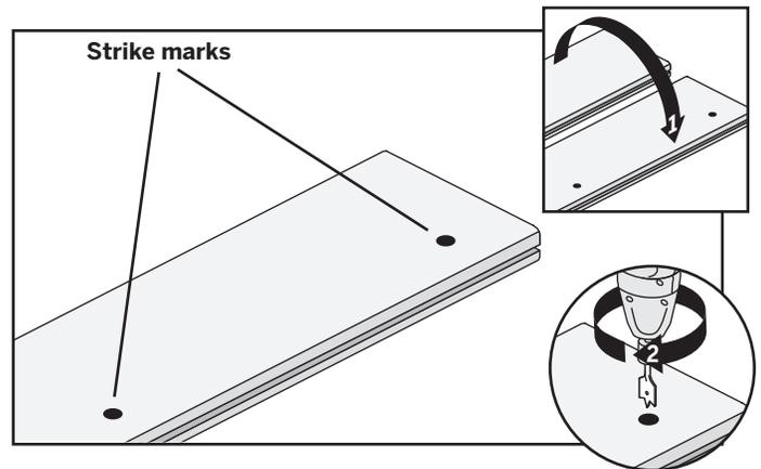
2. Flip board over so that bottom of board faces up and shows strike marks from the screws. Using a paddle drill bit, carefully drill holes to the depth of the fastener heads in the joist. Flip board over so that drilled holes fit over joist fasteners, and fasten board per instructions.
