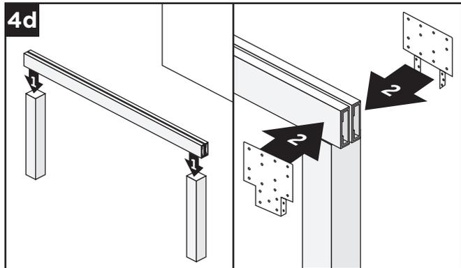
4d. Attach beam to post using NCS front and back beam brackets and required fasteners. See *Required Fasteners* chart on page 6, column A, for approved metal-to-metal fasteners for attaching brackets to beam.
