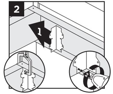
3. Notch outer rim track to allow for fit over end of ledger. Attach outer rim track with metal-to-metal screws (see *Required Fasteners chart on page 6, column A*) every 12" (30.5 cm) top and bottom.
