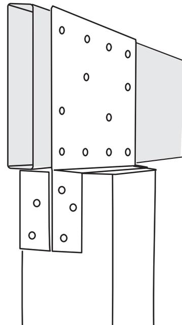
**NOTE:** The post must be pre-drilled to attach beam bracket.
