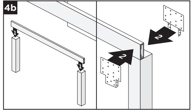
4b. Attach beam to post using NCS front and back beam brackets with required fasteners. See *Required Fasteners chart on page 6, column A, for approved metal-to-metal fasteners for attaching brackets to beam.*
