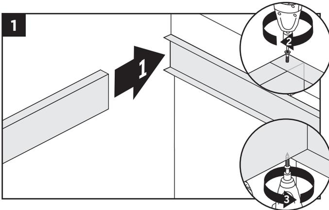
1. Slide the joist within the flanges of the track and rest the outer end on the support post or beam. Fasten joist to track using required fasteners. See *Required Fasteners chart on page 6, column A*. Fasten through the track flange into the joist on top and bottom.
