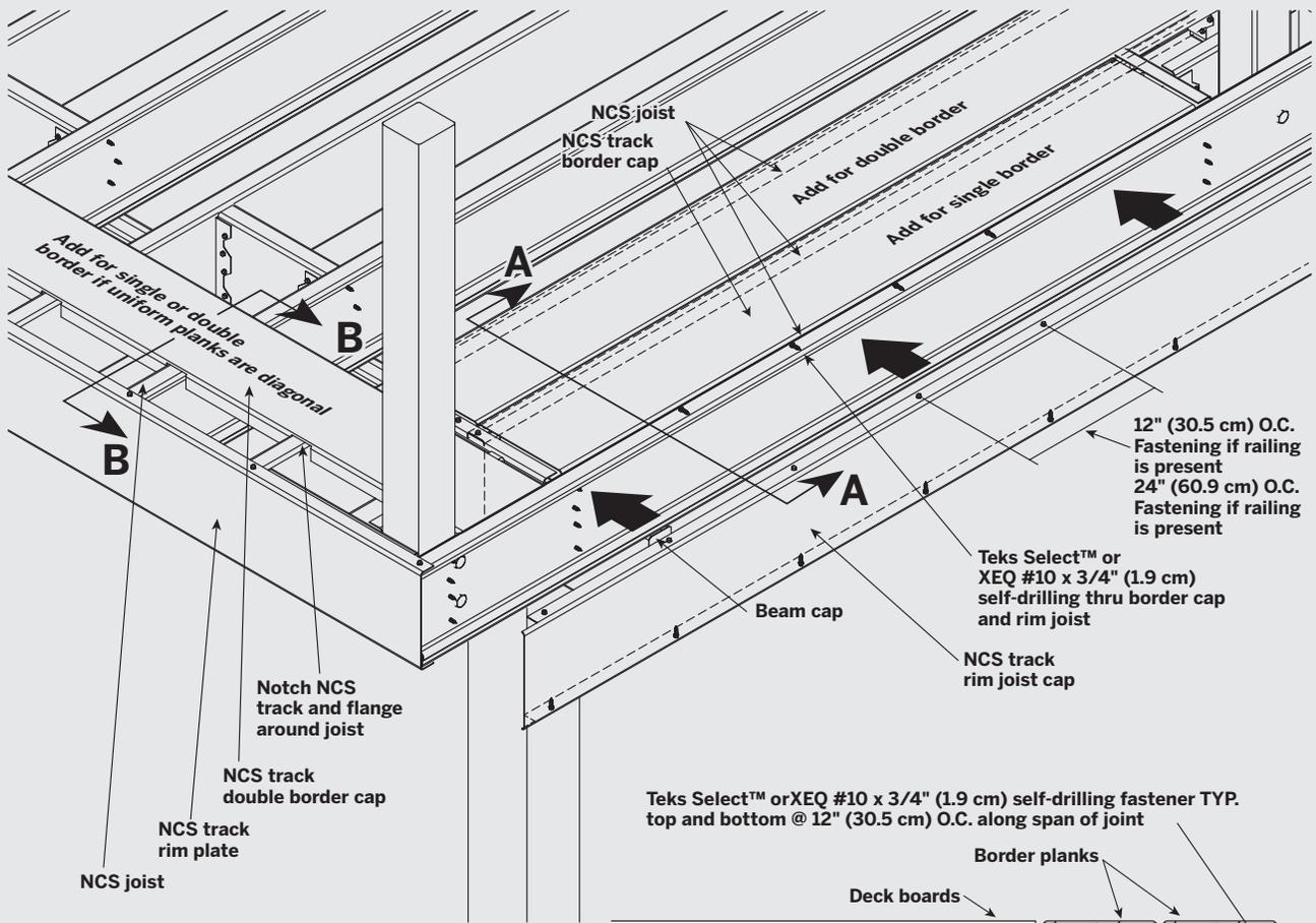
Teks Select™ or XEQ #10 x 3/4" (1.9 cm) self-drilling fastener TYP. top and bottom @ 12" (30.5 cm) O.C. along span of joint
