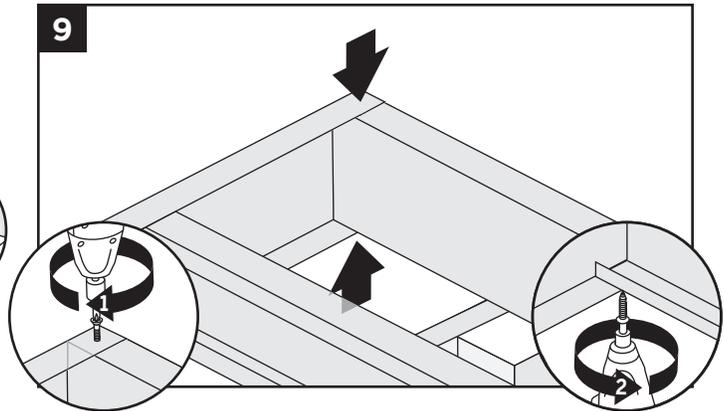
9. Attach track to joists by screwing track to joists in the corners on the top and bottom using required fasteners. See *Required Fasteners chart on page 6, column A*.
