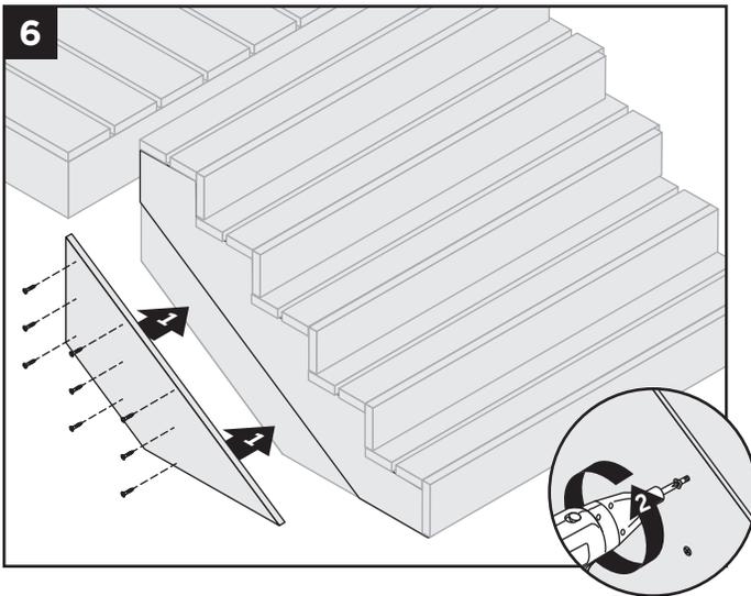
6. Fasten second fascia board (two 1x8 fascia boards are needed in most cases, as one fascia board will not cover stringers) to stair framing by screwing recommended decking with metal fasteners into the stair framing. Number of screws used would depend on width of fascia, if full 1x8 is used, three screws would be required. See *Required Fasteners chart on page 6, column B*.
