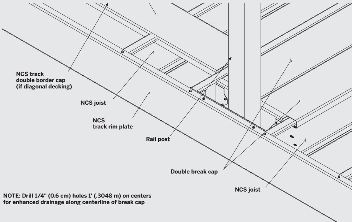
NOTE: Drill 1/4" (0.6 cm) holes 1' (.3048 m) on centers for enhanced drainage along centerline of break cap
