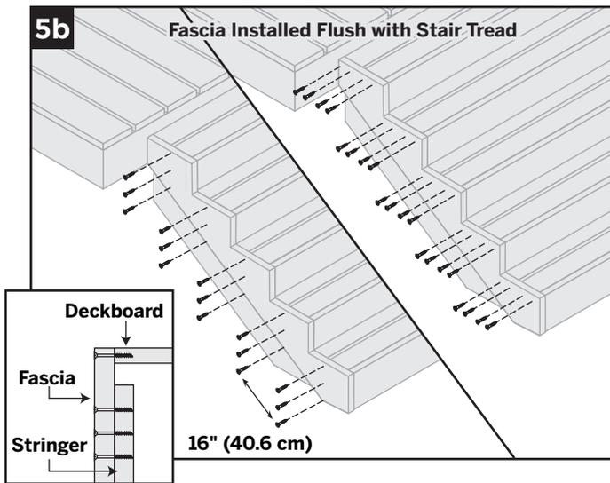
5b. Fasten fascia boards to deck boards from the side as shown. Three fasteners are required every 16" (40.6 cm) for fascia into stringer and two are required to attach fascia into each deck board. See *Required Fasteners chart on page 6, column B*.
