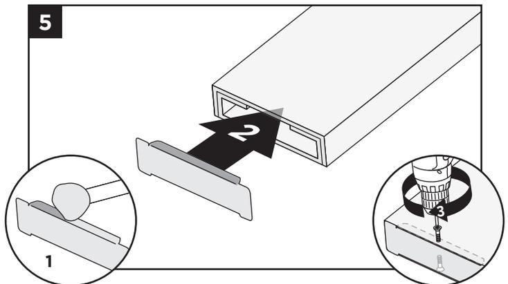
5. Secure cap with exterior grade metal adhesive and/or #10 x 3/4" (1.9 cm) self-tapping screws.
